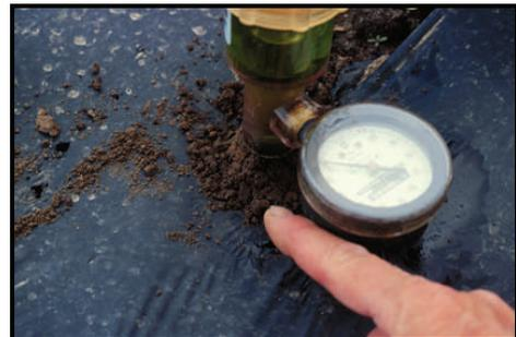
**Figure 5.** Firm the soil around the base of the tensiometer so that rain water does not run down the side of the tube and distort your reading.
