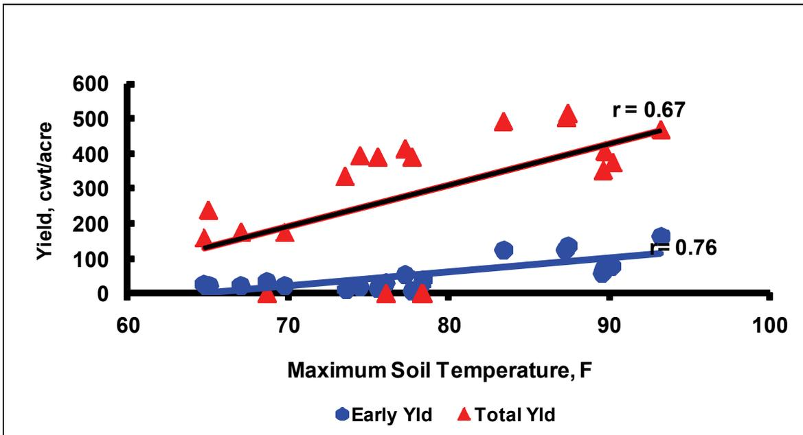
**Figure 4.** Polyethylene mulch effect on tomato yield as a result of 4-inch soil temperature, from 1997 to 2001 studies, Iowa.
