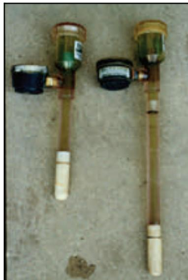
**Figure 11.** 6-inch and 12-inch tensiometers with vacuum gauges and ceramic cups.
