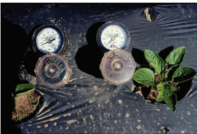
**Figure 2.** The gauge on the left indicates a drier condition (higher reading) than the gauge on the right (a low reading, less than 10 cbar).
