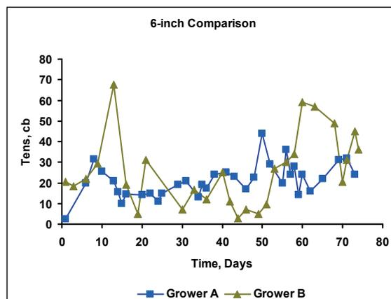
**Figure 13.** Two growers' ability to maintain the 6-inch tensiometer reading between 20 to 25 cbars for a high tunnel tomato crop.
